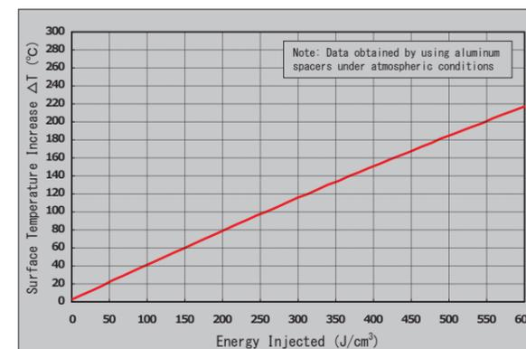
Fig. 23: Relationship Between Energy Injected and Surface Temperature Increase
