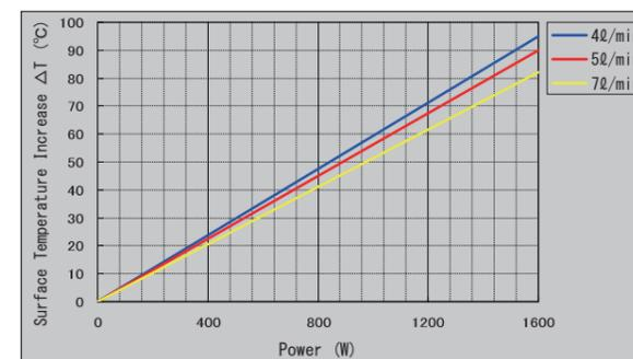
Fig. 20: Surface Temperature Increase vs. Power (W-1600DN)
