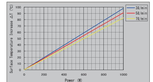
Fig. 19: Surface Temperature Increase vs. Power (W-1000DN)
