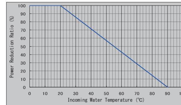
Fig. 14: Derating Curve for Direct Water-Cooled Resistors
