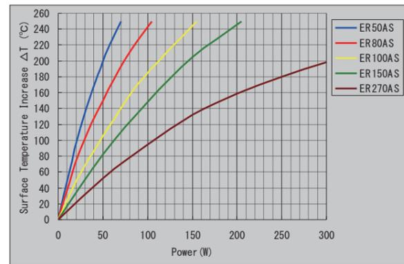
Fig. 5: Surface Temperature Increase vs. Power for AS (2)
