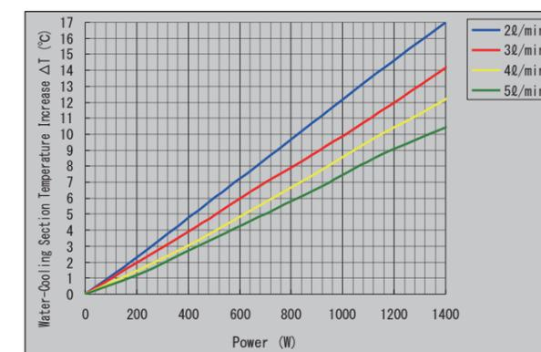
Fig. 28: Water-Cooling Section Temperature Increase vs. Load Power by Water Flow Rate (WD-2)
