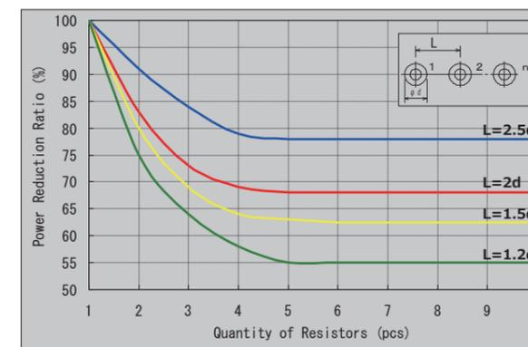
Fig. 2: Power Derating with Resistors Combined
