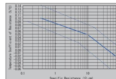
Fig. 13: Temperature Coefficient of Resistance vs. Specific Resistance (room temperature to 200°C)
