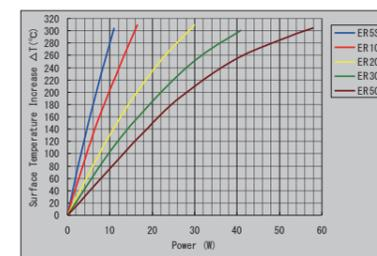
Fig. 10: Surface Temperature Increase vs. Power (1)
