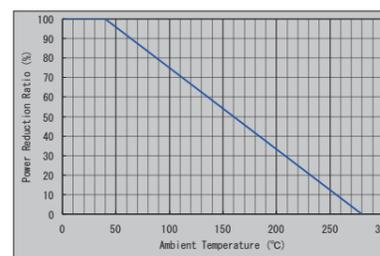
Fig. 9: Derating Curve
