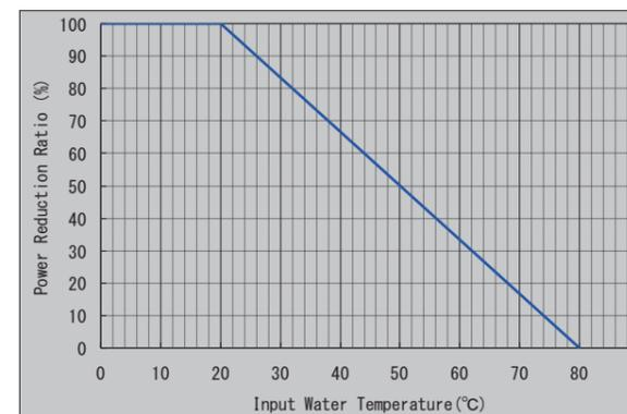
Fig. 25: Derating Curve
