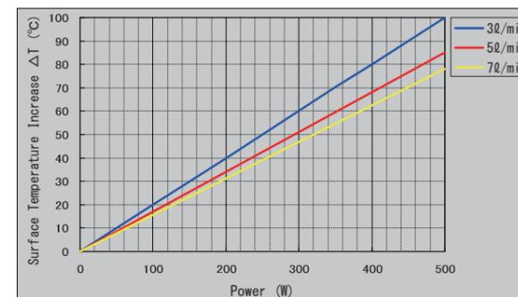
Fig. 18: Surface Temperature Increase vs. Power (W-500DN)
