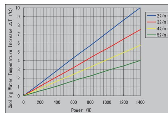
Fig. 27: Cooling Water Temperature Increase vs. Load Power by Water Flow Rate (WD-2)
