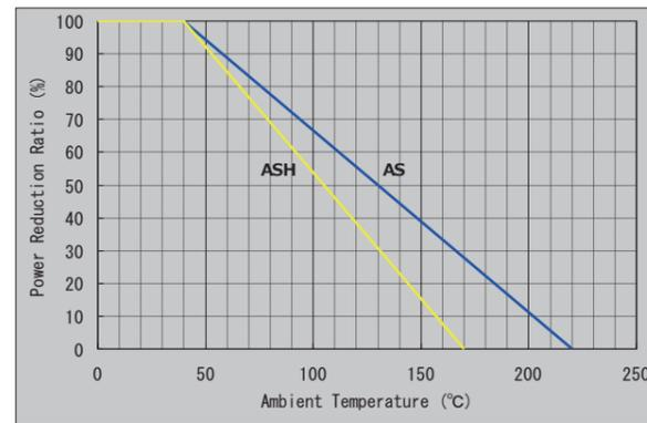
Fig. 3: Derating Curves for AS and ASH
