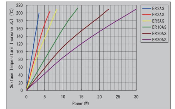
Fig. 4: Surface Temperature Increase vs. Power for AS (1)
