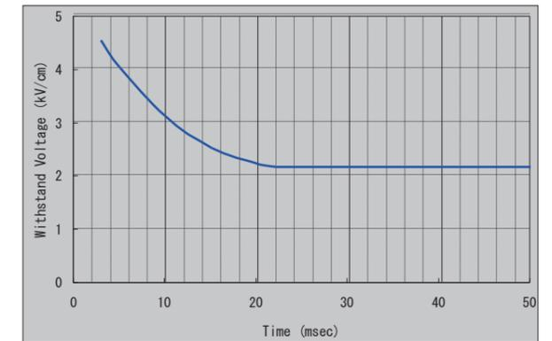
Fig. 22: Withstand Voltage vs. Time
