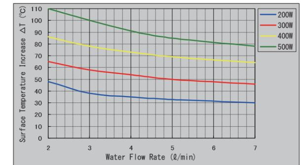
Fig. 15: Surface Temperature Rise vs. Water Flow Rate Curves (W-500DN)
