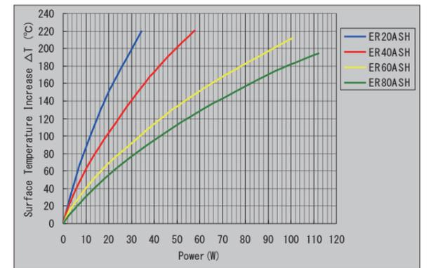
Fig. 6: Surface Temperature Increase vs. Power for ASH
