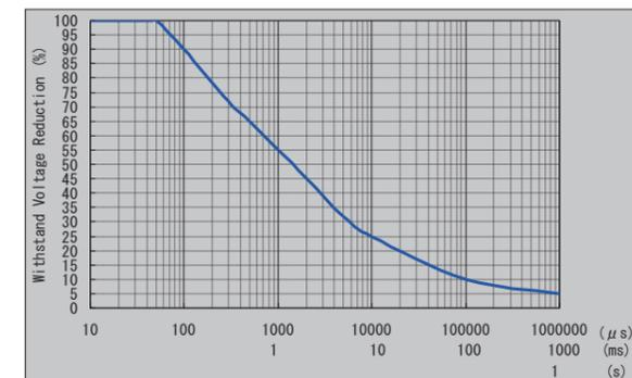
Fig. 1: Voltage Reduction with Impulse Waveform
