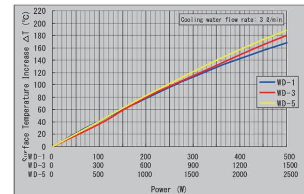
Fig. 26: Surface Temperature Increase vs. Load Power
