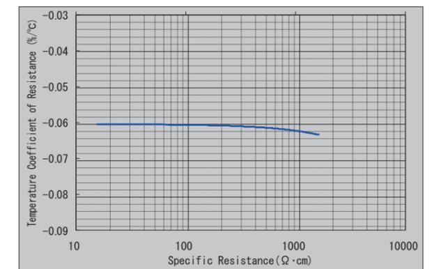
Fig. 24: Temperature Coefficient of Resistance vs. Specific Resistance (room temperature to 200°C)
