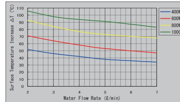
Fig. 16: Surface Temperature Increase vs. Water Flow Rate (W-1000DN)
