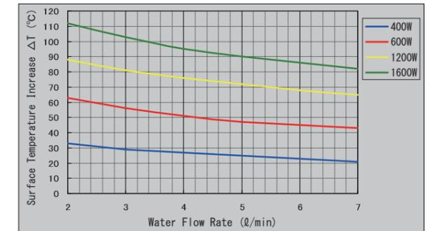
Fig. 17: Surface Temperature Increase vs. Water Flow Rate (W-1600DN)
