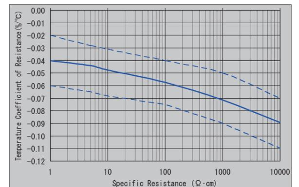
Fig. 8: Temperature Coefficient of Resistance vs. Specific Resistance (room temperature to 200°C)
