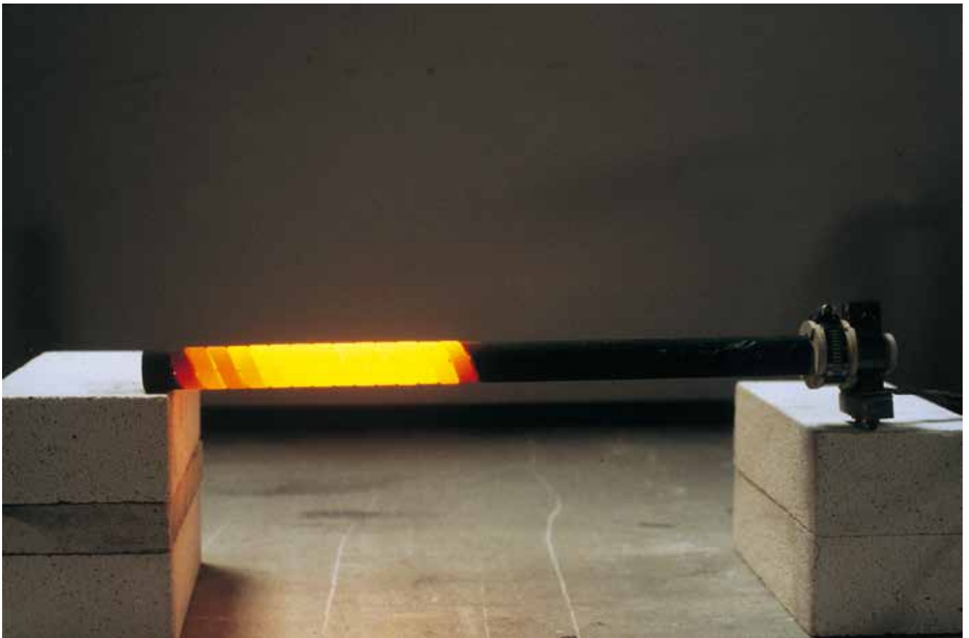
■ Fig. 2 Comparison of types SG and SGR with type E (Test conditions 1600°C in open air)
