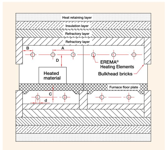
■ Fig. 13 Installing space of heating elements
