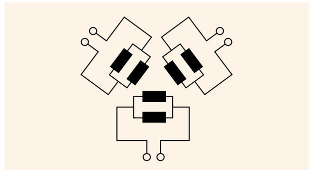
■ Fig. 20 Open delta connection (single phase 3 circuits)
