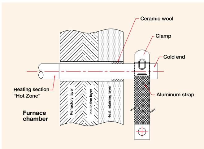
■ Fig. 12 Installation with a terminal clamp
