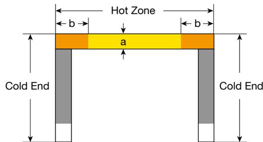
Standard length of the low temperature area (b) shall be 1.5 times of the heating element diameter (a).
