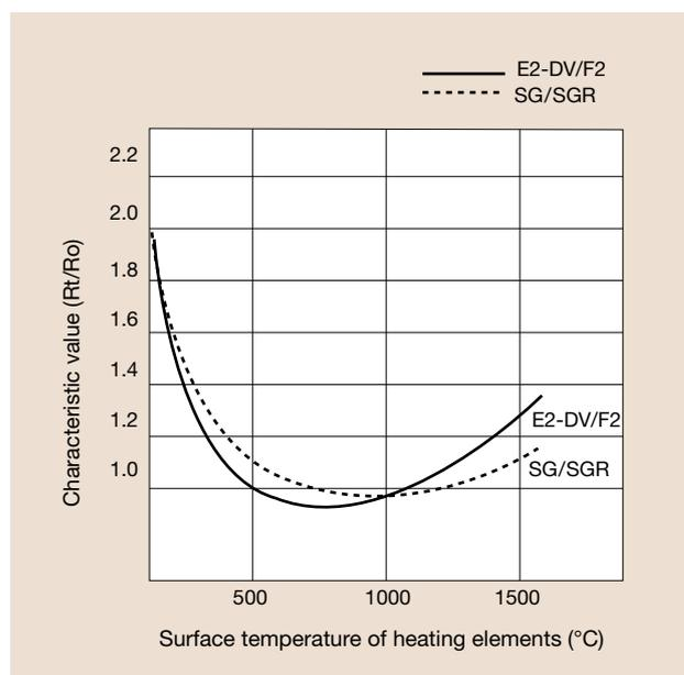
■ Fig. 1 Characteristics of resistance and temperature
