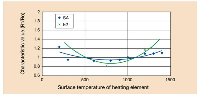
■ Fig. 3 Resistance-temperature characteristics of the SA type
