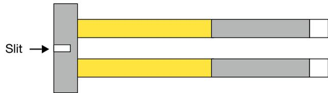
Type U7 has a slit at the center of the crossbar.
